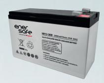
HR (High Rate) series Valve Regulated Lead Acid (VRLA) battery is designed for heavy load discharge applications with 8 years design life in float service. By using strong grids, thick plate and specially designed active material. It is with lower I.R, lower self discharge rate, high power, and longer service life. The HR series battery offers 30% more power output than the standard series. It is suitable for high power standby used, such as datacenter, UPS, EPS etc.
