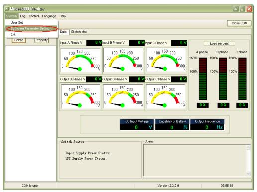
◆A window of "Software Parameter Setting" comes out as below, COM choose according to the UPS, baud rate choose 9600, protocol choose "modbus", then save this setting.
