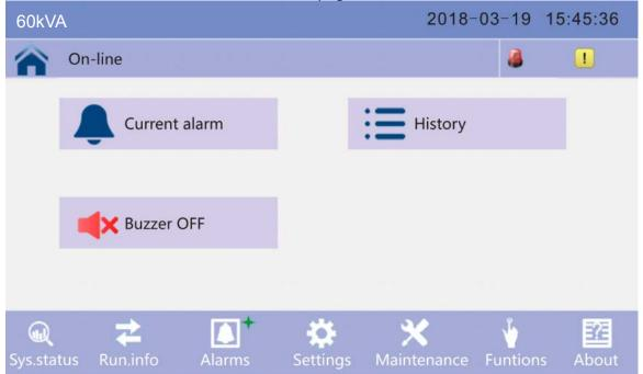
1) Click on the active Alarmicon to enter the module data window, can see the alarm data, click on the back icon return to last windowand click on the homepageicon jump to main page.
