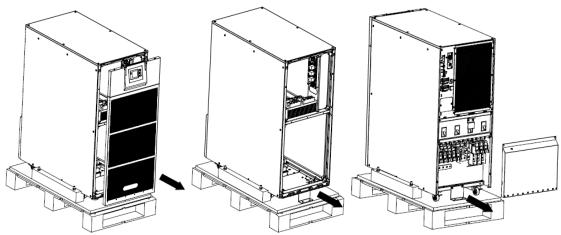
**Step 8**Remove the front panel and real panel to remove the L-shaped bracket and the plates at the left and right side of the UPS that secures the cabinet and the pallet, and secure the sliding
