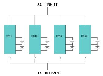
Make sure each UPS input breaker is in "off" position and there is no any output from each UPS connected. Battery groups can be connected separately or in parallel, which means the system itself provides both separate battery and common battery.
