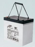
HR ( High Rate ) series Valve Regulated Lead Acid (VRLA) battery is designed for heavy load discharge applications with 15 years design life in float service. By using strong grids, thick plate and specially designed active material. It is with lower I.R, lower self discharge rate, high power, and longer service life. The HR series battery offers 30% more power output than the standby used, such as datacenter, UPS, EPS etc.
