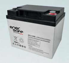
HR (High Rate) series Valve Regulated Lead Acid (VRLA) battery is designed for heavy load discharge applications with 15 years design life in float service. By using strong grids, thick plate and specially designed active material. It is with lower I.R, lower self discharge rate, high power, and longer service life. The HR series battery offers 30% more power output than the standard series. It is suitable for high power standby used, such as datacenter, UPS, EPS etc.
