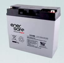
The HR (High Rate) series Valve Regulated Lead Acid (VRLA) battery is designed for heavy load discharge applications with 8 years design life in float service. By using strong grids and specially designed active material the HR series is with lower I.R, lower self discharge rate, high power, and longer service life performance. Generally the HR series offers 30% more power output than the standard range. Suitable for high power standby and cycling situation, such as UPS, datacenter,
