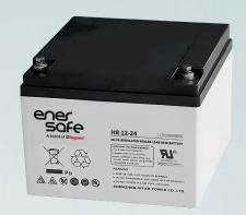
The HR (High Rate) series Valve Regulated Lead Acid (VRLA) battery is designed for heavy load discharge applications with 8 years design life in float service. By using strong grids and specially designed active material the HR series is with lower I.R, lower self discharge rate, high power, and longer service life performance. Generally the HR series offers 30% more power output than the standard range. Suitable for high power standby and cycling situation, such as UPS, datacenter,
