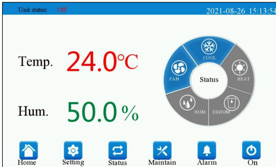
Fig. 1-3-1 Micro-processing controller panel
