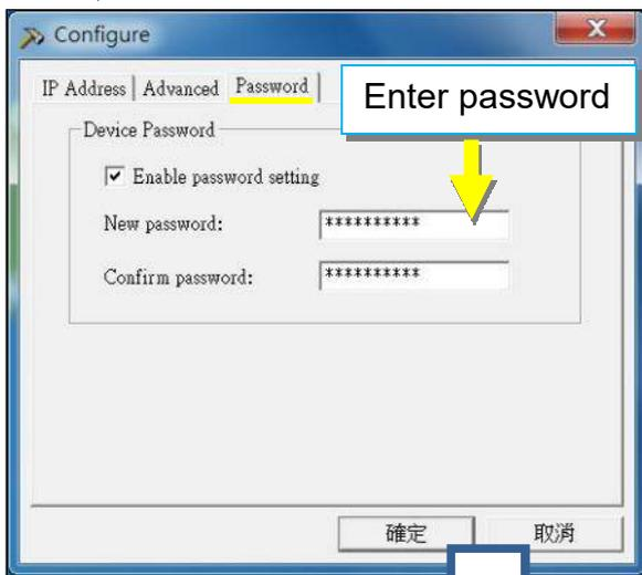
Once password is enabled and configured, it is required to enter the correct password when change any setting or firmware upgrade
